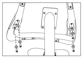
Figure 8: Installing the handlebars
